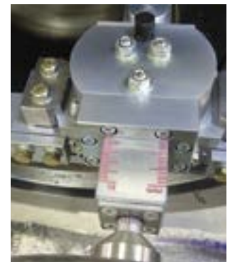
Modules are clearly marked to indicate depth and prep angle
