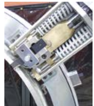
OD tracking slides follow out-of-round pipe & vessels.
