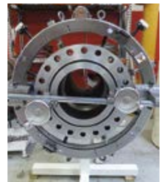
Two FFR modules performing simultaneous operations
