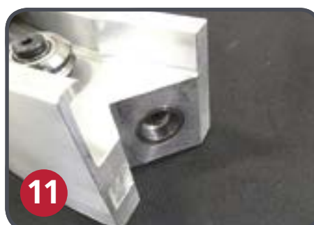
Patent pending V Lock ring mating surfaces are easier to join & stronger
