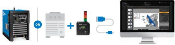
Insight Centerpoint collects welding parameters such as voltage, amperage, wire-feed speed and gas flow.
