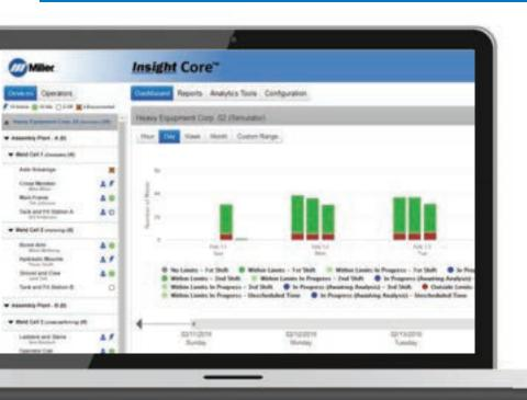
Do you know whether your company's welds are within acceptable ranges for amperage, voltage and wire-feed speed? Insight Core can tell you. It can also provide a date and time stamp, including a weld trace, for every weld. You'll have the necessary documentation to identify machines or welders that operate outside of expected parameters — so you can drive continuous improvement of the products you manufacture.
