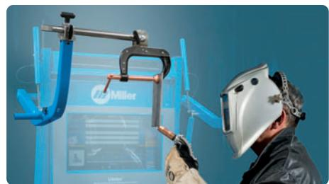
**Welding positioning arm** allows for training in out-of-position GMAW, FCAW and SMAW applications.
